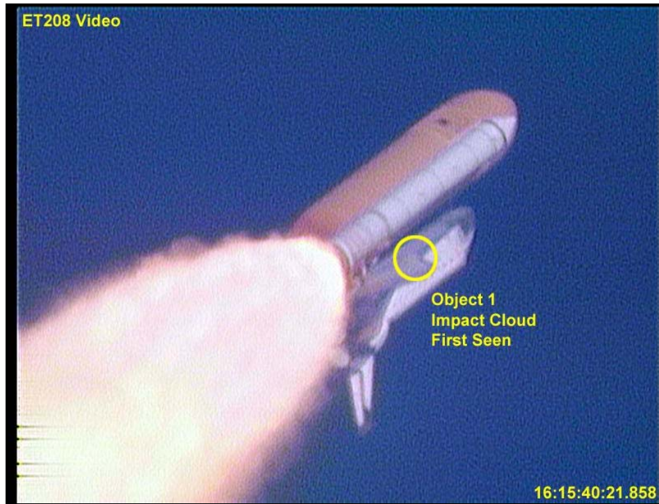
Figure 4.3.2.1b ET-208 View of the debris at 016:15:40:21.858 UTC just after impact with the underside of the leading edge of left wing
