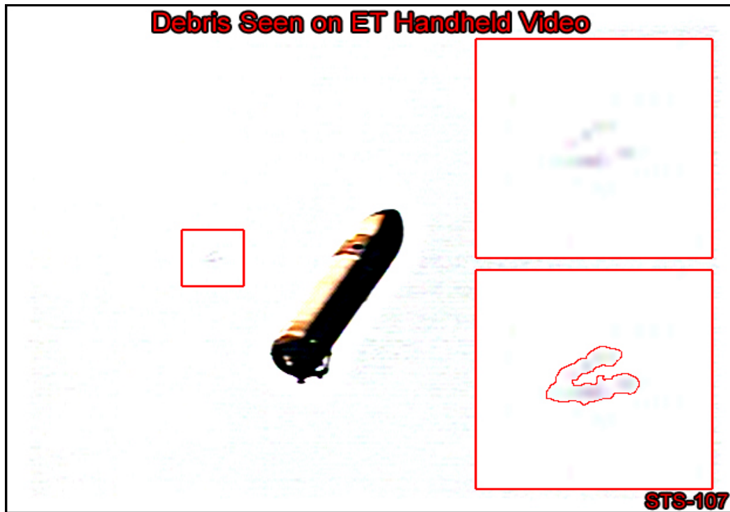
Figure 5.3.1 View from the STS-107 downlink video of the External Tank and the debris, including an enhancement of the debris on the right side of the frame.
